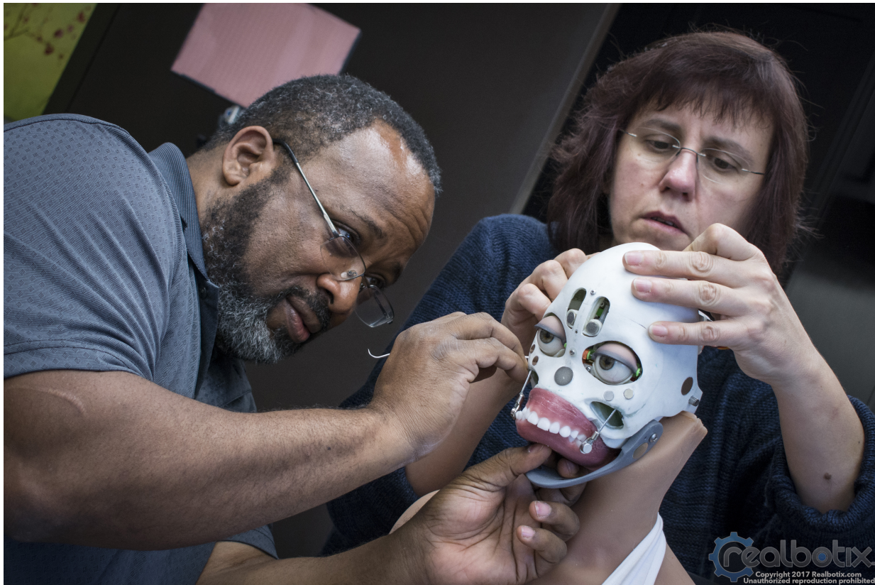
Figure 2: Assembly of the robotic head
