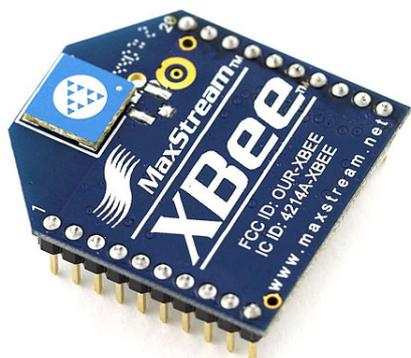
An other solution could be seen in the use of Xbee modules, these small RF transceivers enable direct input and output pins, which enables a 1 on 1 mapping between the transmitter input and the receiver output pins. This in combination with a range of up to 1.6 kilometers if you use the PRO version looked perfect for my application.
