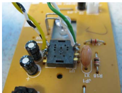
fig. 7 - Wires soldered to pins 3, 4, 6 and 7
