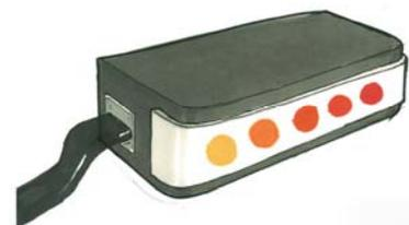
The location of the RJ12 connector and the beams to fix it to a robot were explored briefly. Important aspects were the symmetry of the block when seen from the front and the possibility to stack several blocks. While at first the possibility of connecting several bricks in a daisy chain was explored, this idea was rejected later since a Mindstorms kit would probably have only LED brick due to costs.
