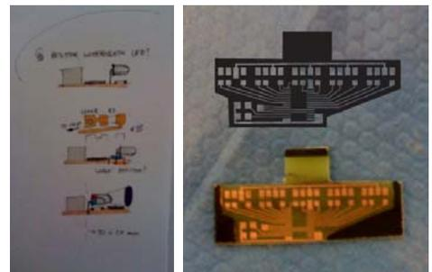
To keep the brick as small as possible and save on soldering wires, a custom PCB was designed using Eagle and Illustrator. After that, the print was made using the laser cutter and etching solution (see image above). *This process will not be described in detail here, if you are interested in knowing more about this process please feel free to contact me.*
