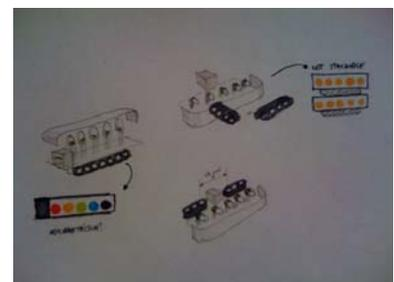
When users want to add several, they can use different ports or have a special connector. The found solution allows for stacking and is symmetrical. Additionally, it is more compact than other solutions.
