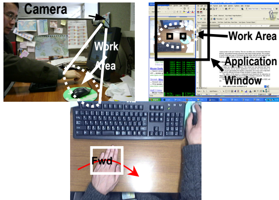
Figure 1. System setup. The camera (left) points at a physical work area on the desktop. The interface image as viewed by the user (middle) can be resized as desired and shows the captured video images and hotspots (right image).
