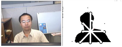
Figure 5. The endpoints of the lines define a polygon used for activity classification.
