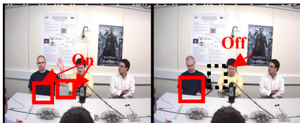
Figure 2. Screen shot of captured image. On the right image a composition of hotspots represents a single command (e.g., re-load a webpage), whereas on the left each hotspot represents a different command (back, forward).
